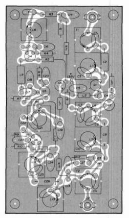
fig. 6. Component layout for the vhf converters. Same circuit board is used for each of the converters shown in figs. 4, 5 and 6. Circuit board is  $2^{1/2}$ " (6.5cm) wide and  $4^{1/2}$ " (11.5cm) long.
